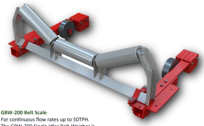
The GBW-200 Single Idler Belt-Weigher is designed to remove high tare loads by using counterbalance weights allowing the use of smaller load cells when weighing very light materials.
