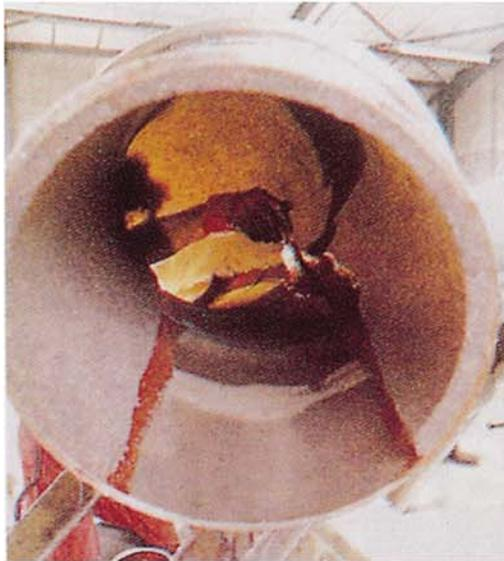
Abrasive wear is one of the greatest problems to be overcome by the maintenance engineer in power stations, coal preparation plants and many other industrial situations where abrasive materials are handled.
